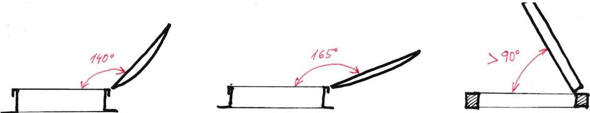
In case of double-flap NSHEV, the final  $C_v$  value can also be slightly increased by setting the opening angle correctly.
